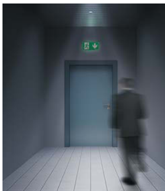
Illustration of the pictograph with a luminance level of 2 cd/m 2
