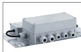
**Connector set (IP65) for outdoor areas** The connector set combines the 24 V signal and data signal in a single output for up to 12.6 m of HILIO (with a 4 m feed line). With the monochrome LED light line, it is possible to apply dimming signals via a separate PWM control line. RGB luminaires that are controlled by DMX or video signals are connected by a connector set that is available as an accessory.
