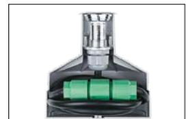
Installation in outdoor areas: a 20 cm thick soakaway underneath the flush-mounted housing drains off ground water. Connection to the supply voltage is obtained outside the casting surround in suitable junction boxes.
