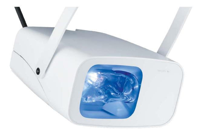
Housing made of die-cast aluminium with high-grade matt white powder coating (RAL 9016); IP65 protection, excellent protection against corrosion and use of materials that are highly resistant to chlorine make this luminaire suitable for use in wellness areas and swimming pools.
