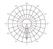
Elliptical light distribution ( $10 \times 20^\circ$ ) guarantees the best possible colour mixing in case of RGB luminaires. Symmetrical light distributions with a beam angle of  $6^\circ$  or  $29^\circ$  meet the various requirements for direct through to indirect illumination.
