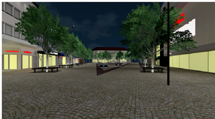
Fig. 22: Variant 1.2 Central with SUPERSYSTEM outdoor 100%, façades 30%, trees 20%, seating cubes 40%, fountain 50%
