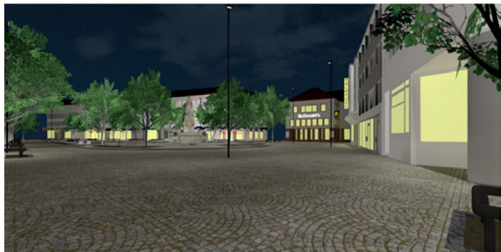
Fig. 30: Variant 1.2 Side with SUPERSYSTEM outdoor 100%, façades 30%, trees 20%, seating cubes 40%, fountain 50%
