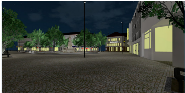
Fig. 29: Variant 1.1 Side with SUPERSYSTEM outdoor 100%, façades 6.5%, trees 20%, seating cubes 40%, fountain 50%
