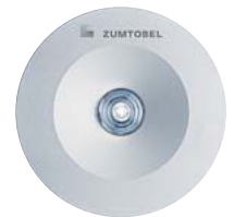
RESCLITE spot LED emergency luminaire for display lighting according to EN 1838. Maximum display lighting: Ø up to 3 m > 5 lux
