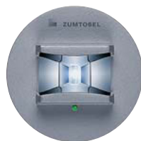
RESCLITE escape LED emergency luminaire for escape route lighting according to EN 1838. Maximum luminaire spacing: up to 23 m > 1 lux
