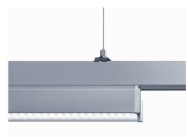
Also in terms of installation, the continuous-row LED lighting system is more convenient and saves time: while previously it was necessary to install the batten luminaire, the reflector and the light source on the trunking one after the other, Zumtobel'sTecton LED is now available as an "all-in-one" solution. All that is now required is for the LED batten to be simply clicked onto the trunking – installation completed! To facilitate individual
