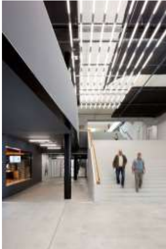
Fig. 3: The aim of the lighting concept is not to produce uniform brightness, but to have the luminaires arranged so as to divide the space into zones and create a dialogue between light and dark.
