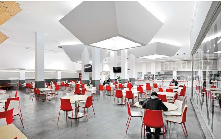
In the windowless cafeteria, the lack of daylight is compensated for by a customised lighting solution incorporating three skylights.
