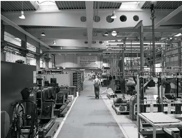
Bosch Rexroth, Pasching | AT Before the lighting was refurbished, employees complained of excessively low illuminance levels, multiple shadows and strobing
