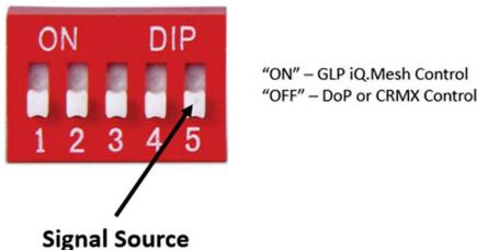
DIP Switch 1 to 4 have no function on this fixture version.
