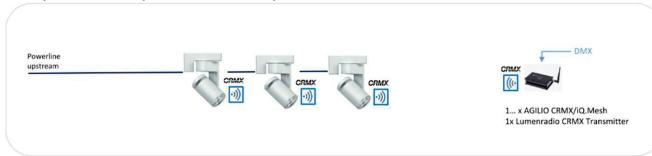
Example with multiple power lines on one single power phase, multiple fixture and one Lumenradio CRMX Transmitter:
