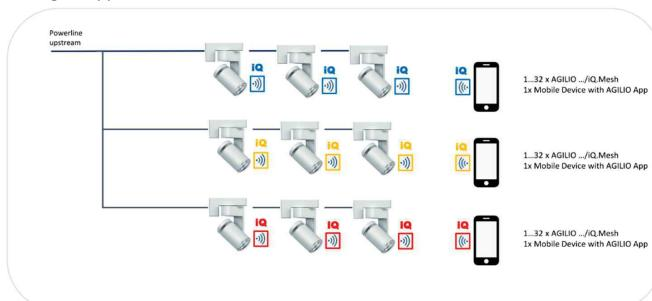
Example with multiple power lines on different power phase, multiple fixtures and one Mobile Device with Agilio App:
