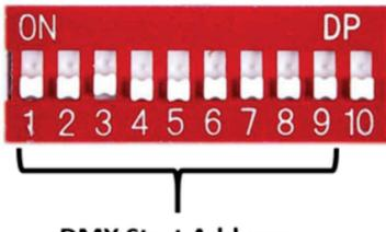
Note that the switches are using a binary coding. We suggest to use a DIP Switch App on your mobile device to quickly calculate the correct switch setting.
