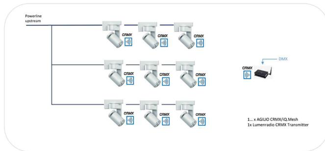
Example with multiple power lines on one single power phase, multiple fixture and multiple Lumenradio CRMX Transmitter:
