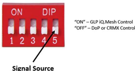
DIP Switch 1 to 4 have to function on this fixture version.
