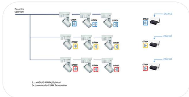
Example with multiple power lines on different power phase, multiple fixture and one Lumenradio CRMx Transmitter:
