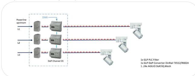
**Note:** The Agilio track adapter can only be contacted with the 3rd power rail of the 3-phase Power Track.
