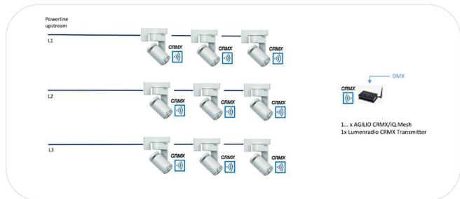
**Note:** The Agilio track adapter can only be contacted with the 3rd power rail of the 3-phase Power Track.
