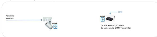
Example with one power line, multiple fixture and one Lumenradio CRMX Transmitter:
