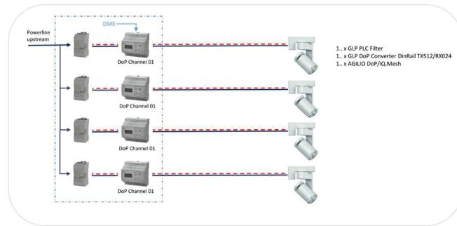
Example with multiple power line on one single phase, multiple fixtures and with ending power distribution. The different DoP lines are decoupled from the power infrastructure on the input side but not decoupled from all other DoP Lines:
