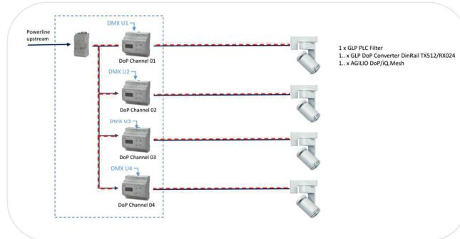
Example with multiple power line on different power phases, multiple fixtures and with ending power distribution. Each separate DoP line is decoupled from the power infrastructure on the input side and decoupled from all other power phases and DoP Lines:
