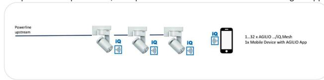
Example with multiple power lines on one single power phase, multiple fixtures and one Mobile Device with Agilio App:
