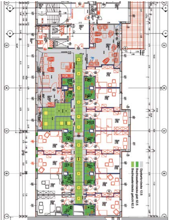
Fig. 4-3. Layout and reflected ceiling plan of the residential ward for dementia patients in the St. Katharina old-age home, position of the luminaires in the corridor area.
