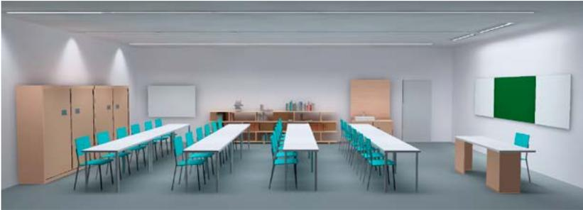
3 x 8m SLOTLIGHT infinity minicell (dimming level 40%) | 2 FEW (dimming level 70%)
