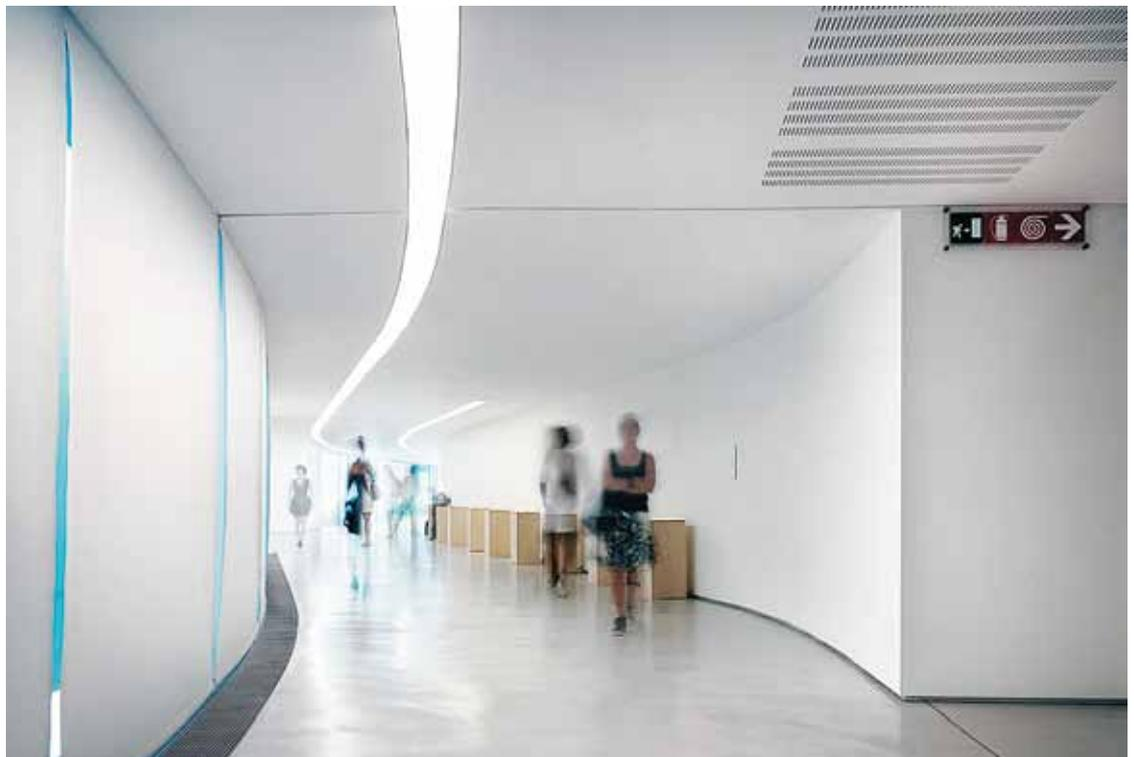
B5 | The lighting is integrated in the ceiling as a continuous light band and also provides an even illumination of the walls.
