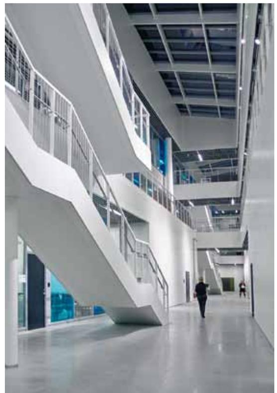
B2 | Most of the building has a specially designed ceiling system with perforated slat-shaped sheet metal segments which also integrates the illumination. Zumtobel won the competition for the best possible fulfilment of the diverse illumination requirements initiated by the client.
