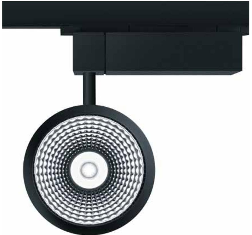
B1 | The sophisticated spotlight design accommodates a unique lens-reflector system. This permits precise and even accent lighting with a range of different light emission characteristics. The special design of the die-cast aluminium housing allows for purely passive cooling of the LED modules, ensuring a long service life.
