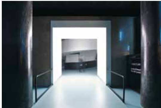
B2 | The exhibition areas are accessible via large illuminated door frames. The portals of light are created using planar light modules – an elegant way to direct visitors to the different rooms, as shown here in the entrance hall.
