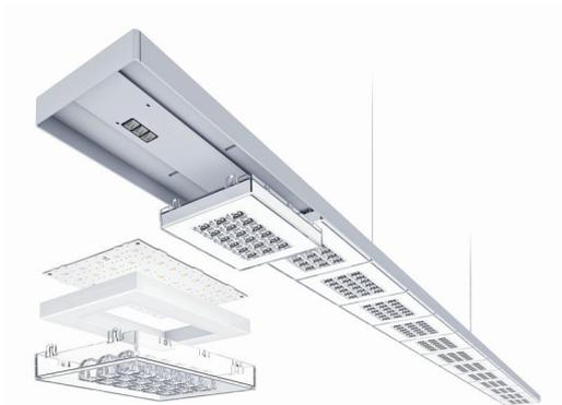
**Caption 2:** Sequence has been designed as a pendant or surface-mounted luminaire and consists of 8 or, optionally, 14 side-by-side module units of identical design, each with 6 x 3 centrally located LED lighting points.
