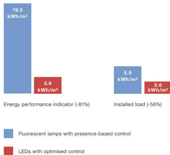
Nevertheless, good economic efficiency of LED luminaires with optimised lighting control in circulation areas cannot be guaranteed in every case despite extremely large, proven power savings. The extra cost of LEDs needs to be approximately CHF 50 to CHF 100 per downlight or per running metre of batten luminaire in order to achieve an amortisation period of 5 to 8 years.
