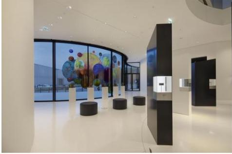
**Fig. 4:** While Zumtobel used PANOS infinity downlights featuring a colour temperature of 3000 K for general lighting, the wallwashers required a colour temperature of 4000 K due to incident daylight.
